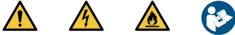
General warning sign ISO 7010 — W001 Warning: Electricity ISO 7010 — W012 Warning: Flammable material ISO 7010 — W021 Refer to instruction manual/booklet ISO 7010 — M002
